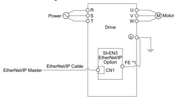
Figure 5.28 Option Connection Diagram
