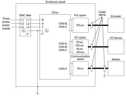
Figure 14.1 Option Installation for CE Compliance: 1000-Series, GA700, GA800, CR700, CH700
