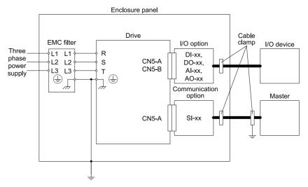
Figure 14.3 Option Installation for CE Compliance: FP605
