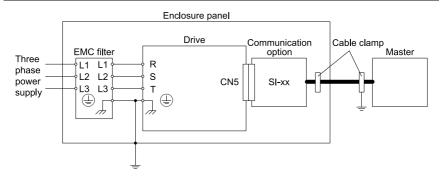
Figure 14.2 Option Installation for CE Compliance: GA500, HV600
