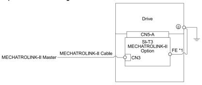
Figure 5.15 Option Connection Diagram
