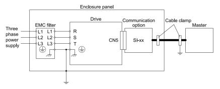
Figure 8.3 Option Installation for CE Compliance with GA500
