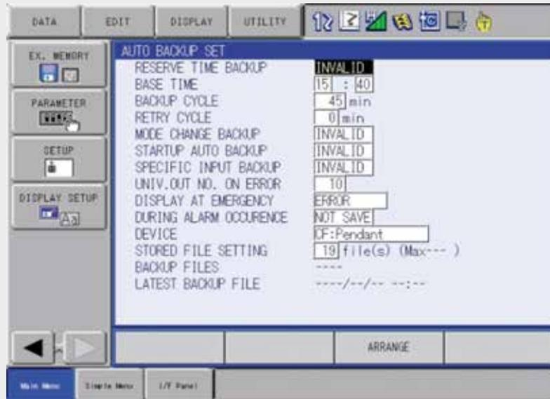
The system data can be collectively backed up so that the data can be immediately loaded and restored in case of an unexpected trouble such as data loss.
