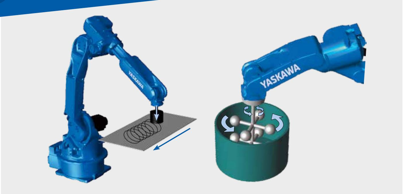
This function continuously rotates the T-axis a plural number of turns. Although the rotation angle of the T-axis is generally limited within  $\pm 360$  degrees, this function allows it to rotate endlessly. When executing the move instruction MOVJ with the "number of rotations of the external axis" specified, the T-axis rotates the "specified rotating amount + teaching position pulses" during the movement to the target position. One move command can specify up to  $\pm 100$  turns.
