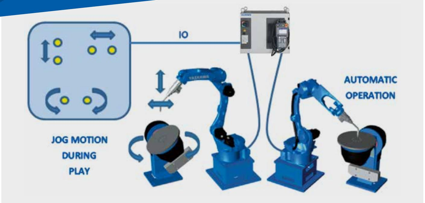
The “I/O JOG Operation in Play-Mode” function performs axis operation for robot and external axes using universal input signals instead of the programming pendant.
