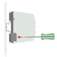
2. The extension module has a locking lever on the upper and lower side. Pull these levers outwards as shown in the figure, until these engage audible.
