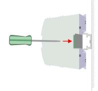
**2.** Each periphery module has a locking lever on its upper and lower side. Pull these levers outwards as shown in the figure, until these engage audible.
