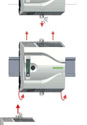
**2.** Remove the CPU with a rotation upwards from the profile rail.
