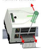
By means of a screwdriver there is the possibility to remove the connectors e.g. for module exchange with a fix wiring. For this each connector has indentations for unlocking at the top. Unlocking takes place by the following proceeding:
