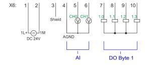
Wiring > Wiring CPU
