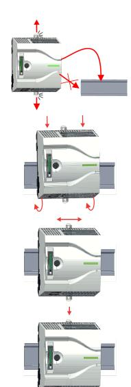
Mounting > Mounting the extension module
