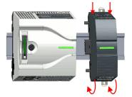
To mount plug the periphery module from the top onto the profile rail and turn the periphery module downward until it rests on the profile rail.
