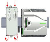
To mount plug the extension module from the top onto the profile rail and turn the extension module downward until it rests on the profile rail.
