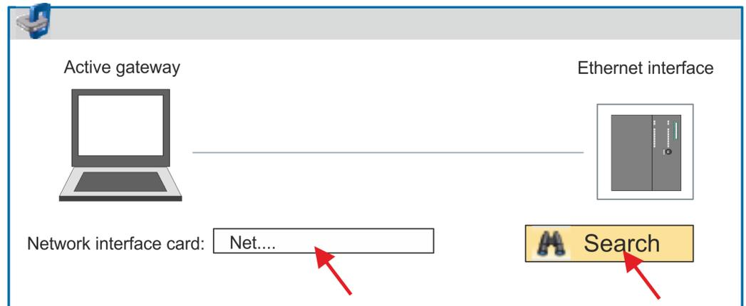
5. Select the according network interface card, which is connected to the Ethernet PG/OP channel and click at '*Search*' to determine the via MAC address reachable device.
