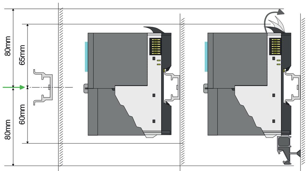
1. Mount the mounting rail! Please consider that a clearance from the middle of the mounting rail of at least 80mm above and 60mm below, respectively 80mm by deployment of shield bus carriers, exist.
