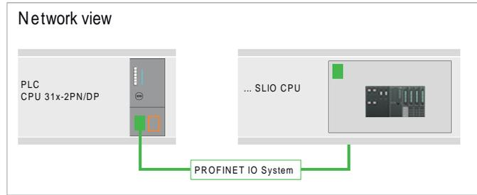
1. After installing the GSDML the 'PN I-Device for ... CPU' can be found in the hardware catalog at 'Other field devices → PROFINET IO → I/O → VIPA ... → ... SLIO System → SLIO I-Device'. Drag 'PN I-Device for ... CPU' from the hardware catalog to Network view.
