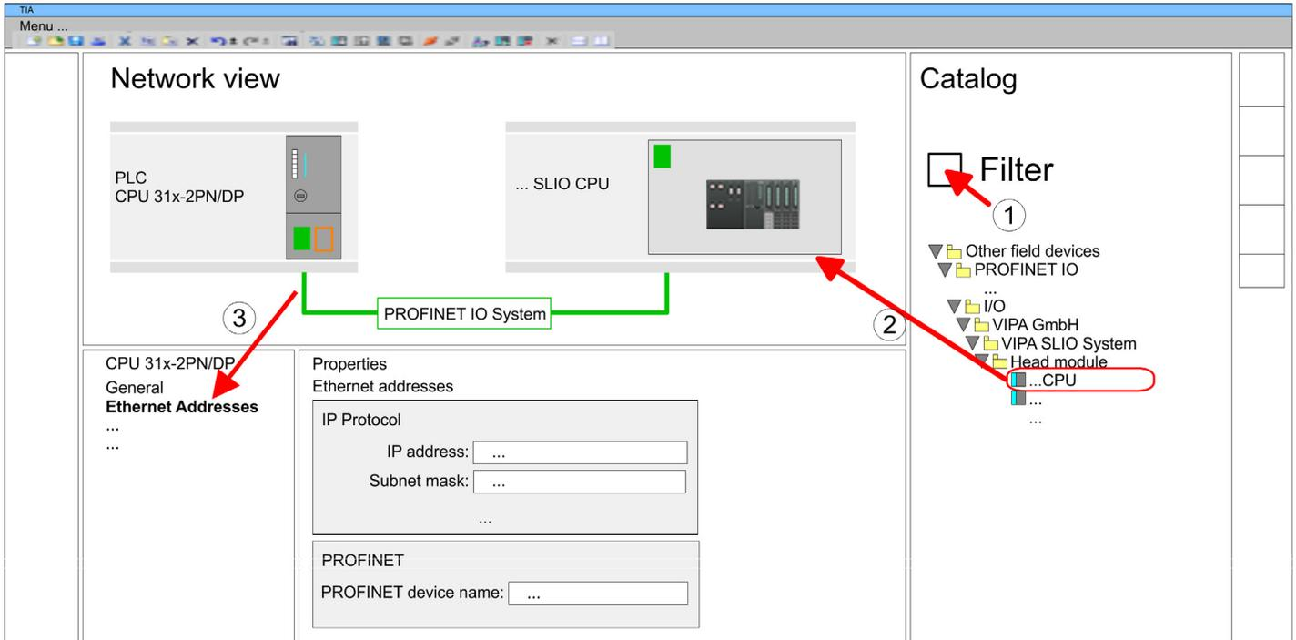
**5.** Select in the *Network view* the IO device '*... SLIO CPU...*' and switch to the *Device overview*.
