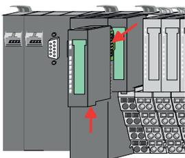
Press the unlocking lever at the lower side of the just mounted right module near the CPU and pull it forward.
