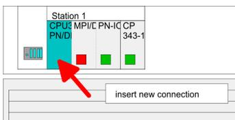
1. ➔ For the project engineering of connections, open the connection list by selecting the according CPU. Choose *Insert new connection* in the context menu:
