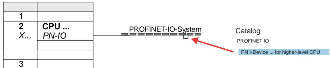
3. ➤ Open the properties dialog by double-clicking System SLIO 'PN-I-Device' and enter at 'Device name' the previously noted name of the I-Device.
