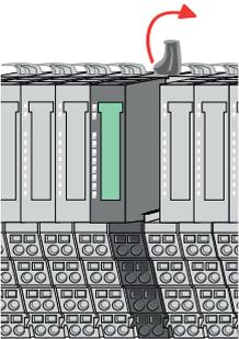
4. ➤ Turn the locking lever of the module to be exchanged upwards.
