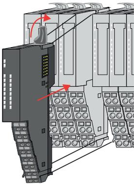
6. ➤ To mount the module put it to the gap between the both modules and push it, guided by the stripes at both sides, to the mounting rail.
