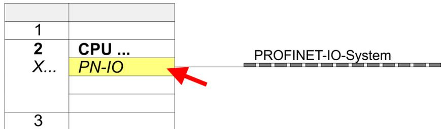
6. ➤ Use [New] to create a new subnet and assign valid IP address data for your PROFINET system.
