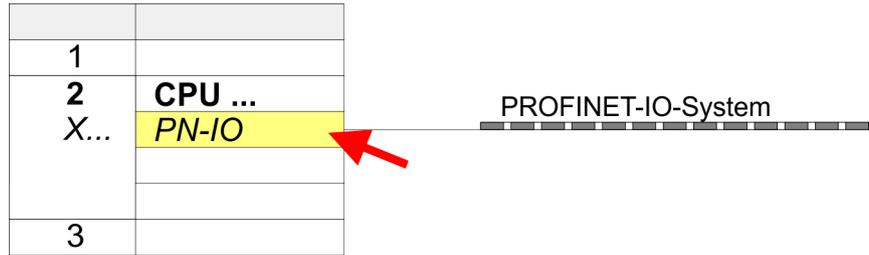
The PROFINET interface of the PROFINET IO controller is parametrized with PN-IO, the port with Port 1. In the following these parameters for PN-IO and Port 1 are described.
