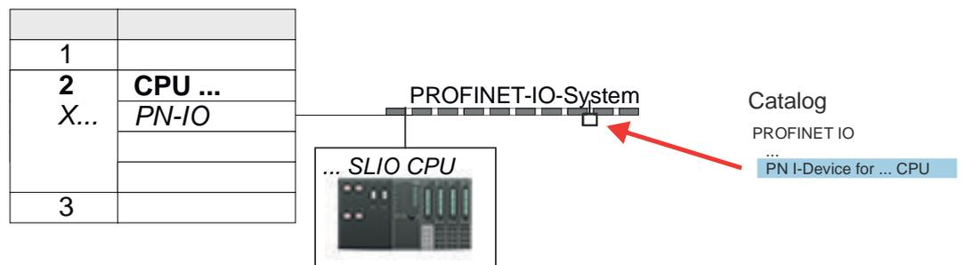
2. ➔ Open the properties dialog of the PROFINET IO controller of the CPU by a double-click at 'PN-IO' and assign a 'Device name' for the I-Device in the Register 'General'.
