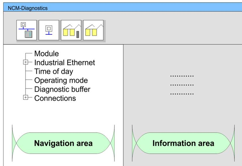
The working surface of the diagnostic tool has the following structure:
