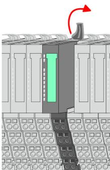
4. ➤ Turn the locking lever of the module to be exchanged upwards.
