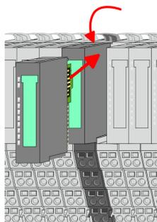
9. Plug again the electronic module, which you have removed before.
