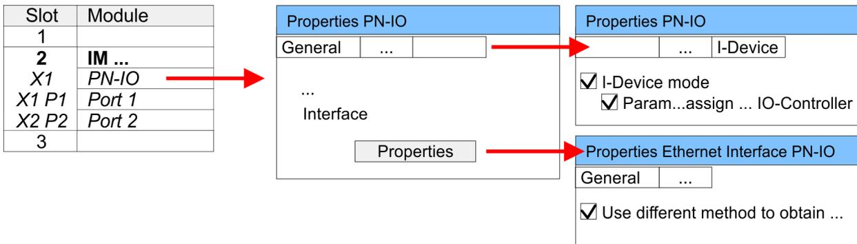
Create an I-Device GSD file and install it at your hardware catalog with *'Options → Create GSD file for I-Device'*. Open the hardware configuration of your higher-level VIPA CPU and connect your Siemens I-Device from *'Preconfigured Stations'*.
