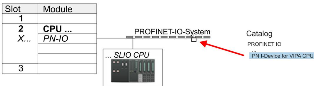
Use as I-Device > Configuration in the Siemens SIMATIC Manager
