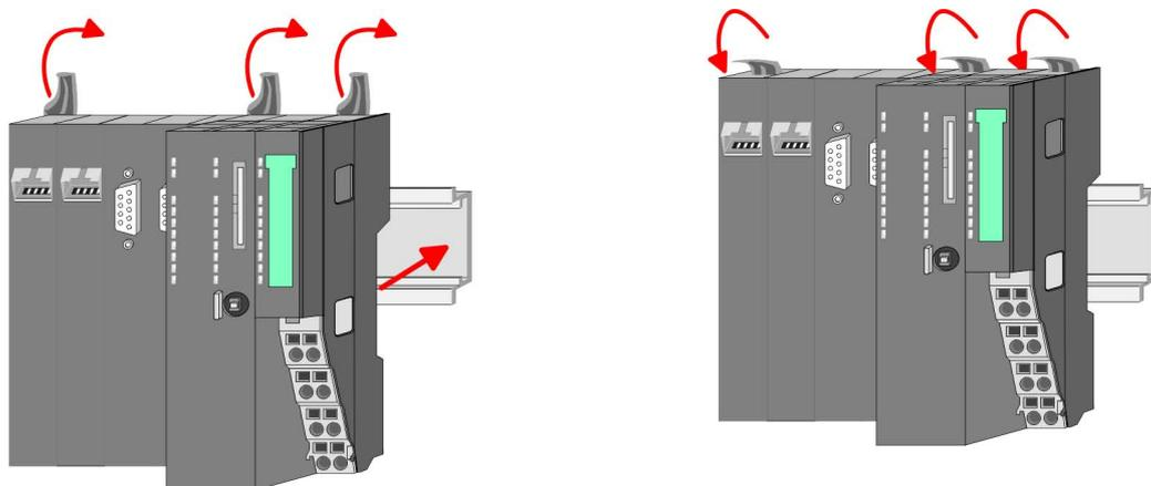
2. Turn the locking lever upwards, place the CPU at the mounting rail and turn the lever downward.
