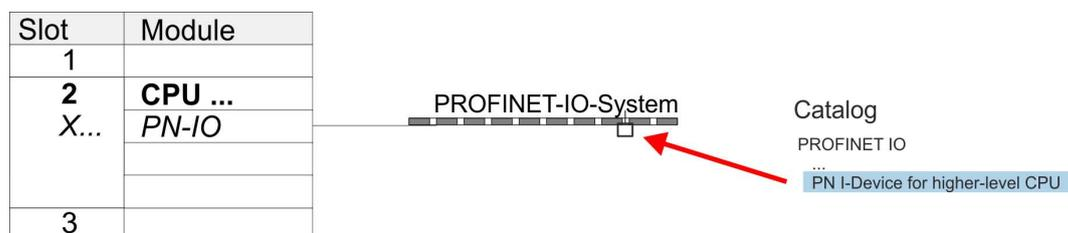
3. ➤ Open the properties dialog by double-clicking 'PN-I-Device' and enter at 'device name' the previously noted name of the VIPA I-Device.
