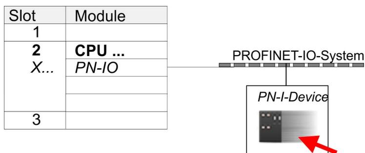
4. ➤ Configure an input area of the same size for each output area of the I-Device in the IO controller and vice versa. Here also no gaps may arise. In particular, make sure that the order of the transfer areas matches that of the I-Device configuration. The following transfer units are available:
