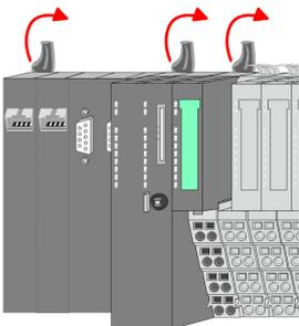
4. Turn all the locking lever of the CPU to be exchanged upwards.
