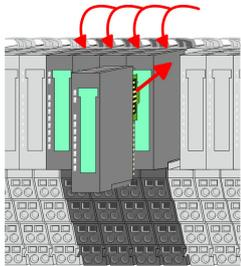
9. ➤ Plug again the electronic module, which you have removed before.
