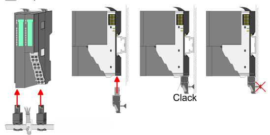
**3.** Attach the cables with the accordingly stripped cable screen and fix it by the shield clamp with the shield bus.
