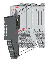
**6.** To mount the module put it to the gap between the both modules and push it, guided by the stripes at both sides, to the mounting rail.
