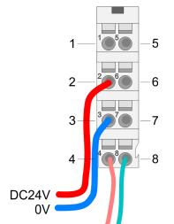
For wires with a core cross-section of 0.08mm<sup>2</sup> up to 1.5mm<sup>2</sup>.
