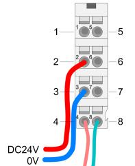
For wires with a core cross-section of 0.08mm<sup>2</sup> up to 1.5mm<sup>2</sup>.
