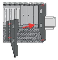
3. After mounting the whole system, to protect the backplane bus connectors at the last module you have to mount the bus cover, now. If the last module is a clamp module, for adaptation the upper part of the bus cover is to be removed.
