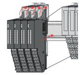
To mount the module group put it to the gap between the both modules and push it, guided by the stripes at both sides, to the mounting rail.
