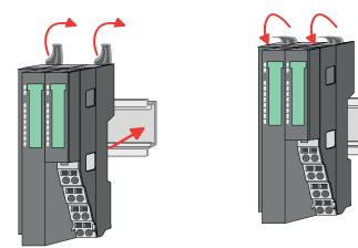
**2.** Turn the locking lever upwards, place the bus coupler at the mounting rail and turn the lever downward.
