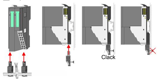
Attach the cables with the accordingly stripped cable screen and fix it by the shield clamp with the shield bus.
