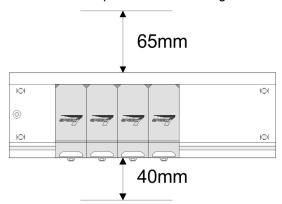
**2.** Connect the profile rail with the protected earth conductor. The minimum cross-section of the cable to the protected earth conductor has to be 10mm<sup>2</sup>.
