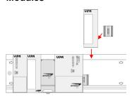
Repeat this procedure with the peripheral modules, by clicking a backplane bus coupler, stick the module right from the modules you've already fixed, click it downwards and connect it with the backplane bus coupler of the last module and bolt it.
