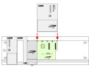
1. To deploy the SPEED7-CPU exclusively at the SPEED-Bus, plug it between the triangular positioning helps to the slot marked with "CPU SPEED7" and pull it down.
