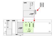
1. If also standard modules shall be plugged, take a bus coupler and click it at the CPU from behind like shown in the picture. Plug the CPU between the triangular positioning helps to the slot marked with "CPU SPEED7" and pull it down.
