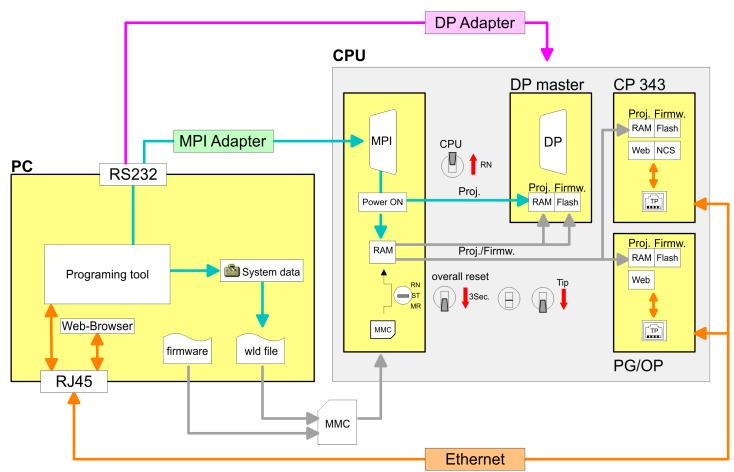
Please always use the **CPU 317-2DP (6EST 317-2AK14 V3.3)** from Siemens of the hardware catalog to configure this CPU from Yaskawa. For the project engineering, a thorough knowledge of the Siemens SIMATIC Manager and the hardware configurator from Siemens is required!
