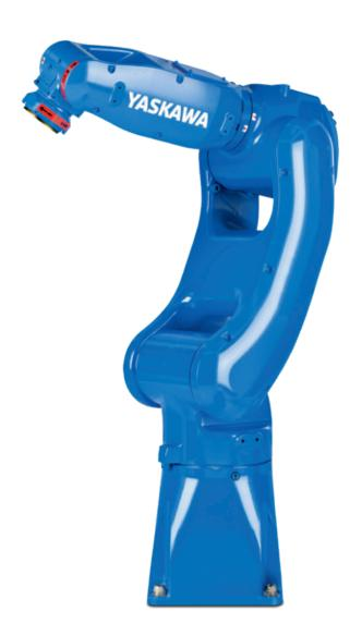
The MOTOMAN GP8 is an extremely fast and precise 6-axis industrial robot with a payload capacity of up to 8 kg. With a reach of 727 mm and a high repeatability of  $\pm$  0.01 mm, it is ideally suited to assembly tasks, but also universal handling tasks, CNC machine tool tending or packaging. Its smooth, streamlined and award-winning modern industrial design is attractive and minimizes the space requirements at the installation site.
